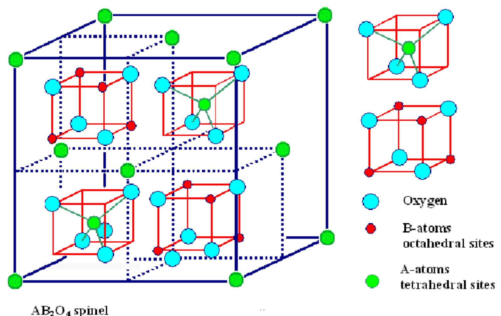
Ferrites are useful absorbers as they are insulating and both magnetically and dielectrically lossy. Transition metal cations occupy octahedral and tetrahedral sites within the lattice. The crystal electric field splits the d orbitals;  $e_g$  orbitals are higher in energy at octahedral sites, and  $t_{2g}$  orbitals are higher in energy at tetrahedral sites.
