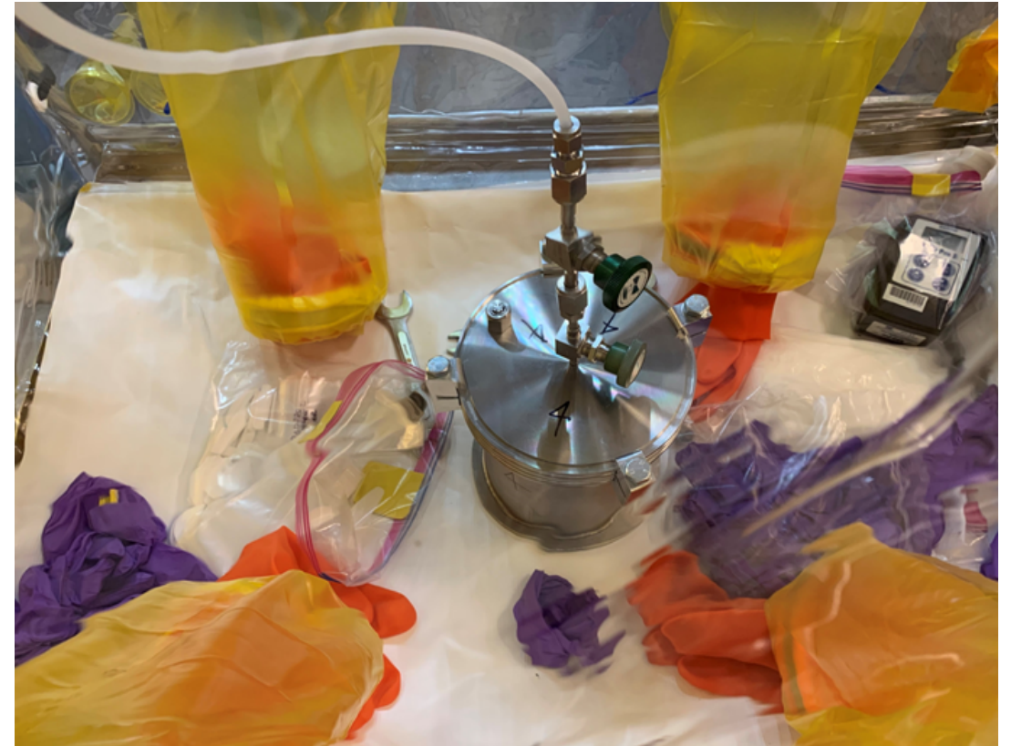
Figure 7. The target transport container and attached vacuum line.
