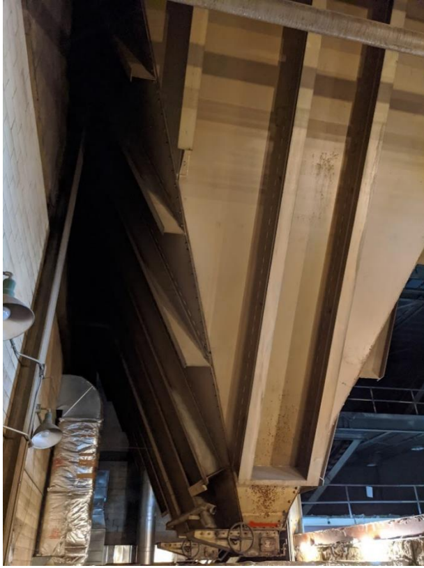
Figure 21. Large steel lined hoppers at the Pilot Plant facility.
