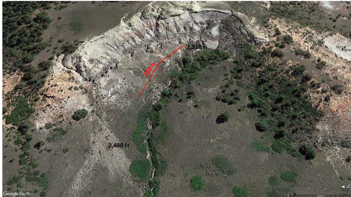
Figure 6. Site Satellite Picture with Expected Required Scoria Trail Layout (red line).
