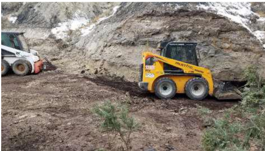
Figure 9. Cleaning of the Coal Seam and Coal Sample Collection.
