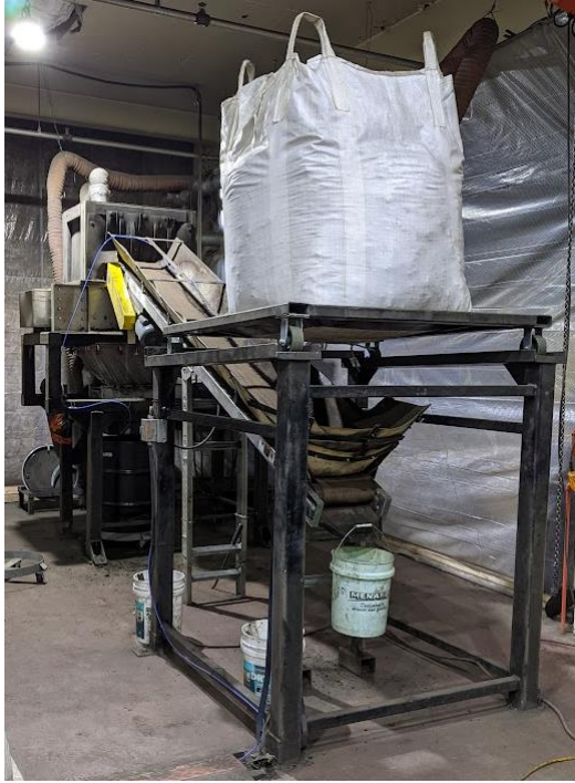
Figure 22. Stacked crushers and supersack unloading stand.
