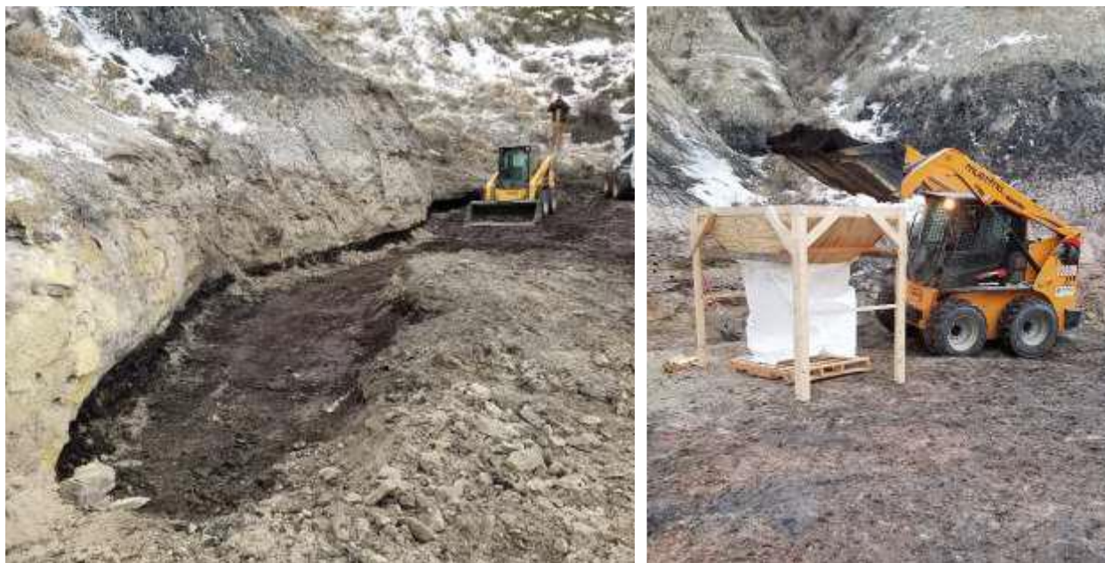
Figure 10. Final Extraction of the Coal Seam and Bagging into Super Sacks.
