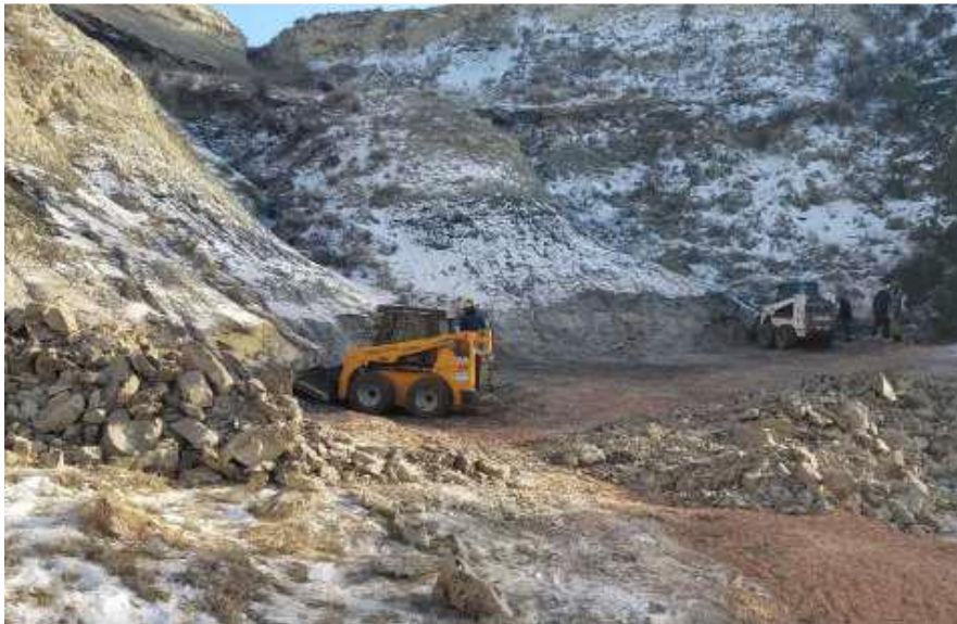
Figure 8. Removal of Overburden Overlaying the Target Coal Seam.
