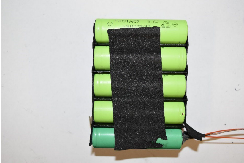
Figure 4. Drill battery setup. Two orange wires are heater power. Tan wire is thermocouple. A hole was drilled in the cell to provide access for a micro-heater and thermocouple.
