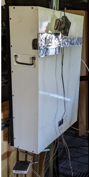
Figure 5. Two directional flame thermometers (DFTs) positioned on the bottom and corner of the battery energy storage system (BESS).
