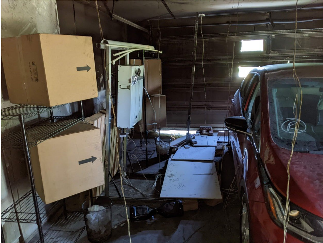
Figure 3. Test fuel configuration. The EV is seen on the right. On the left wall are the BESS, along with several standard combustible items. The three drill batteries in two wastepaper baskets and the hoverboard are on the floor of the garage between the EV and the left wall. An electric vehicle with a 66-kWh NMC 622 battery was in the center of the garage. All batteries except for the EV battery were tested at 100% state of charge (SOC). The EV battery was at 30% SOC.
