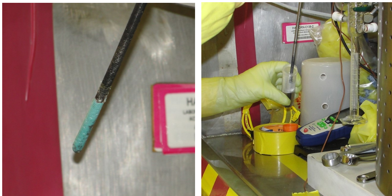
Figure 11. Sample collected on Hastelloy rod being mixed in water.
