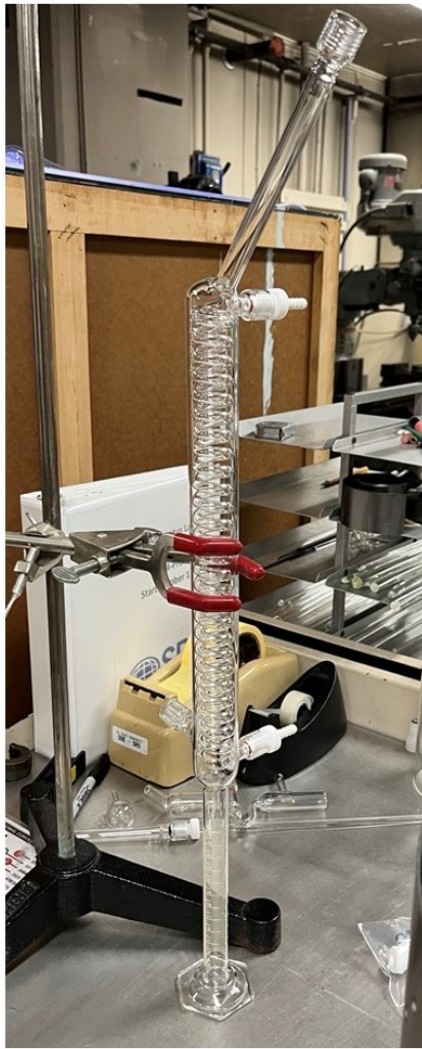
Figure 7. Water-cooled capture condenser that has been modified to measure collected condensates.
