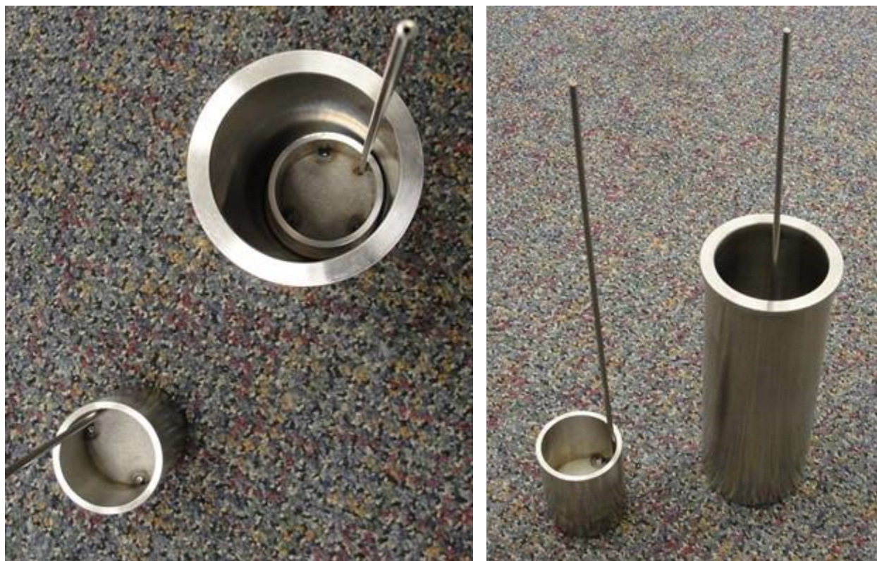
Figure 18. Gas sparger design for Experiment 5 showing the frit sparger and reaction vessel liner.
