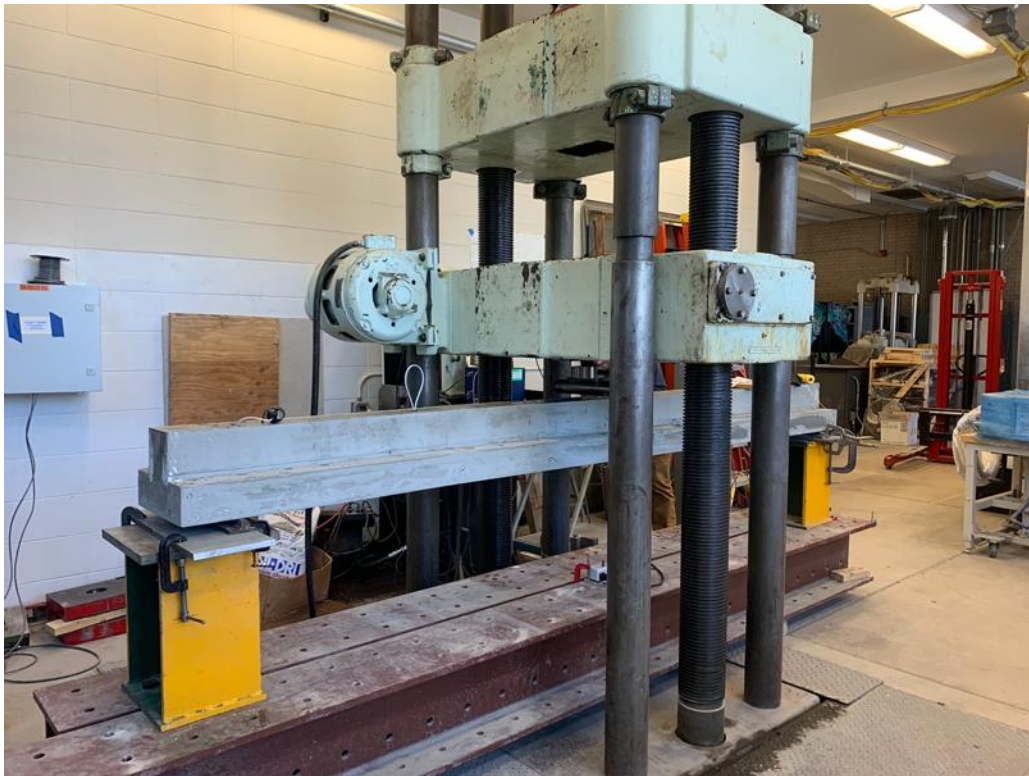
Figure 6 – Photo of an experimental HVFA inverted tee beam installed in the test setup
