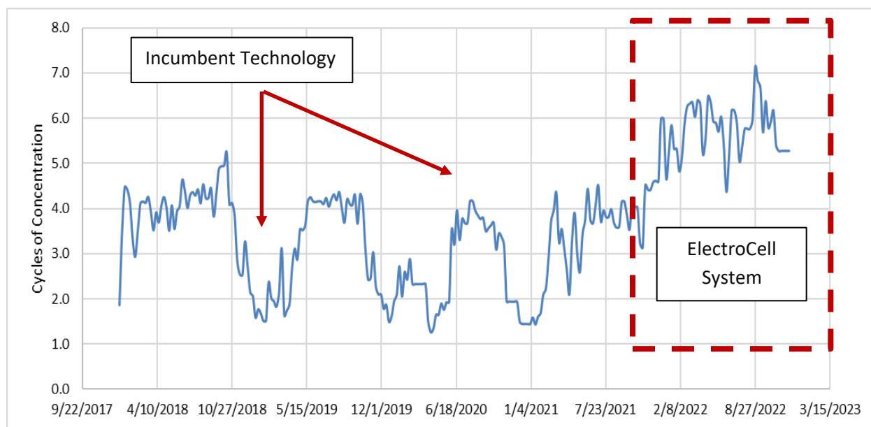
Figure 14. Cycles of concentration (COC), incumbent vs. ElectroCell systems
