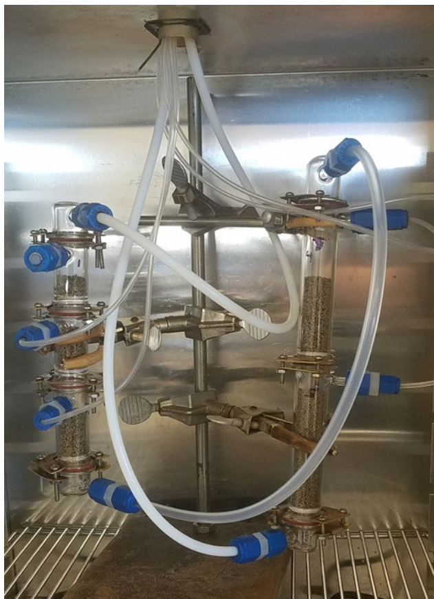
Figure 2-4. Configuration of the sorbent beds inside the temperature-controlled oven.
