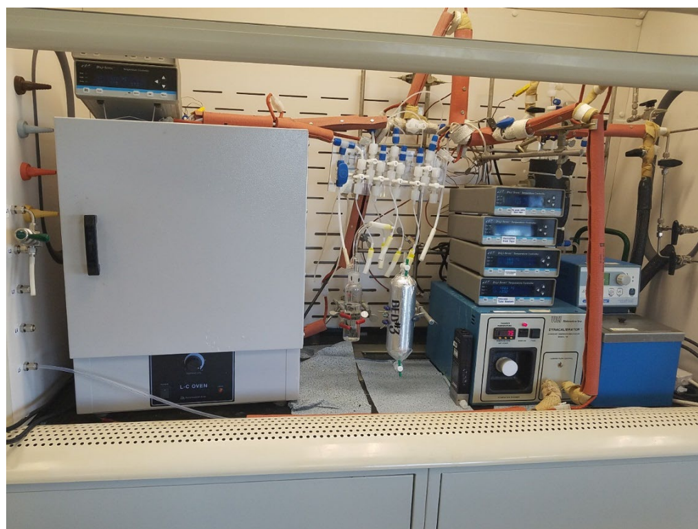
Figure 2-2. Deep-bed adsorption test system inside a laboratory hood. At left: Oven containing the sorbent beds; and middle showing a 100-mL gas scrubbing impinger, and glass sample tube for GC analysis. At right: Thermal control panels on permeation tube oven and humidifier water bath.
