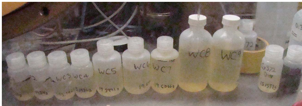
Figure 4-8. Test 3 Yellow Tint of Wash and Displacement Solutions
