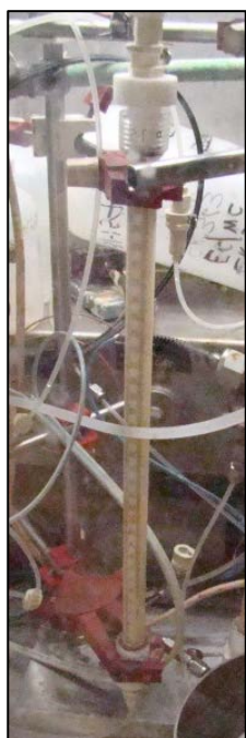
Figure 3-2. Radioactive Anion Exchange Column
