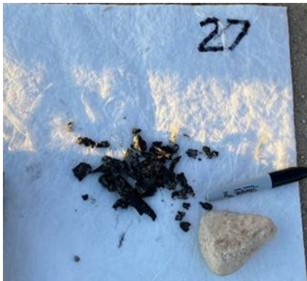
Figure 6. Copperhead plug parts after drill-out operations
