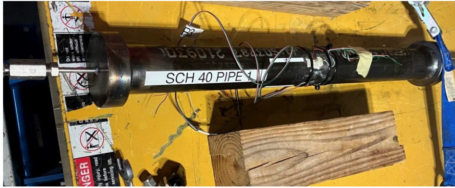
Figure 6. Pressure burst test setup for SCH-40 Pipe 1.
