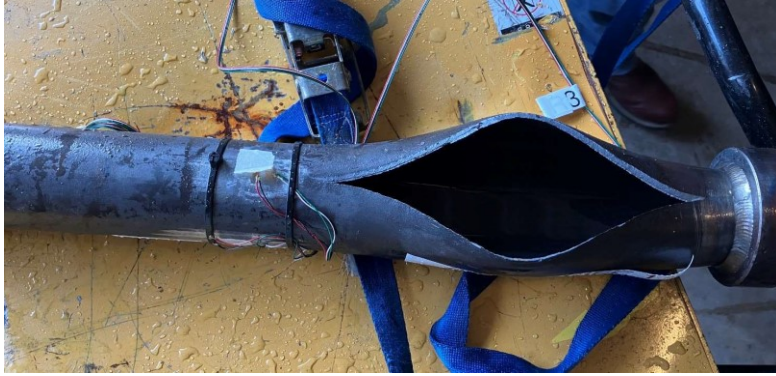
Figure C3. Schedule 80 Pipe 1 after bursting.
