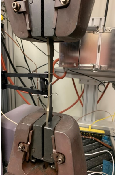
Figure 4. Tensile specimen fixture, extensometer, and broken specimen.
