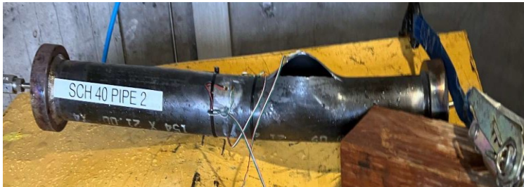
Figure C2. Schedule 40 Pipe 2 after bursting.
