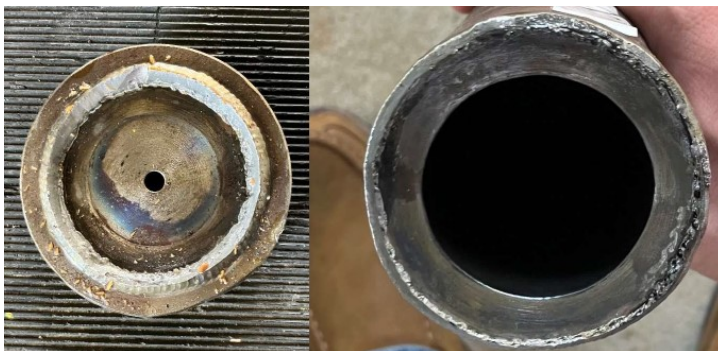
Figure C5. Schedule 160 Pipe 2 after bursting.
