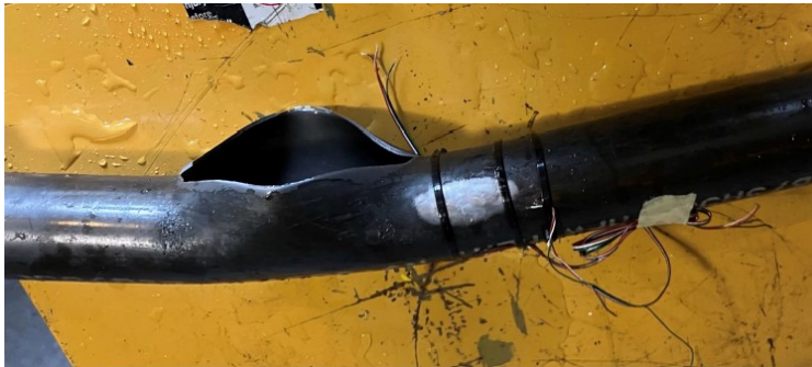
Figure C1. Schedule 40 Pipe 1 after bursting.
