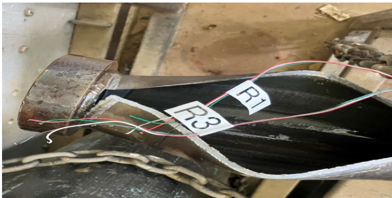
Figure C4. Schedule 80 Pipe 2 after bursting.
