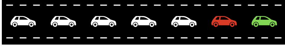
Figure 4.5: Vehicle formation used in simulation. A trajectory leader (in green) driving a speed profile drawn from the dataset is placed in front of an AV (in red) which is followed by a platoon of 5 human vehicles (in white), modeled using the Intelligent Driver Model.
