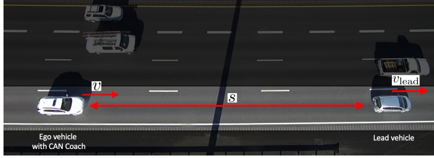
Figure 3.1: Ego vehicle with CAN Coach (White Toyota RAV4) and lead vehicle (Silver Honda Fit) in formation in the right lane.
