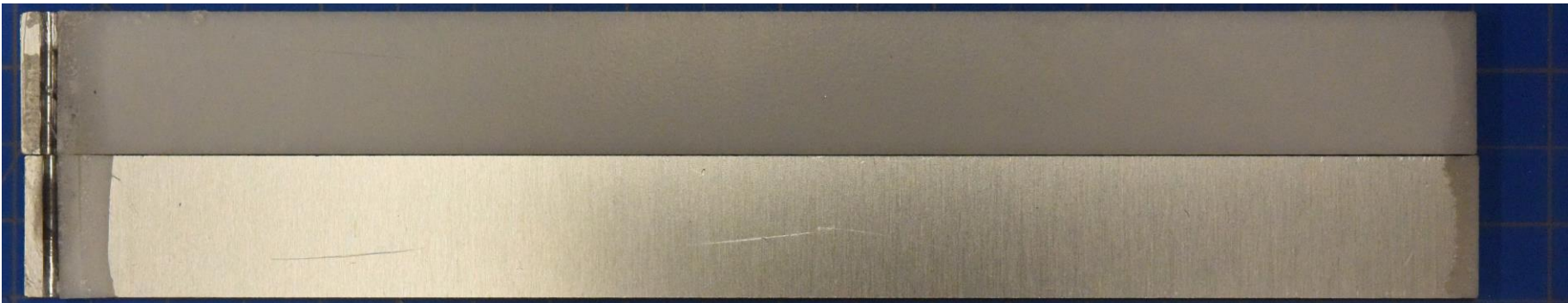
Adhesive failure of 6061-T6/ANA interface for unprimed SAA II w/HWS at -55°C
