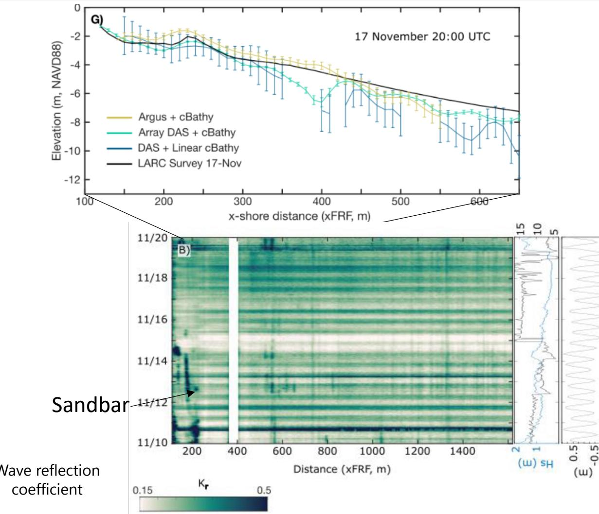
Bathymetry is well captured by applying cBathy to DAS data (array method)
