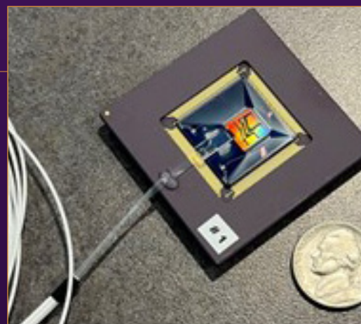
Fig. 1. A prototype lidar sensor utilizing silicon photonics technology developed by Sandia researchers.
