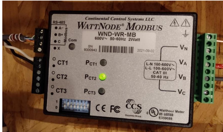
Figure 12. WattNode device used to measure electrical energy consumption of heating system loads including the central blower and the heat pump compressor. A gas submeter was installed to record furnace gas consumption.
