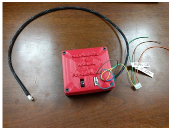
Figure 14 - Dongle that allowed the project's control logic to be implemented on the test site's dual fuel heating system
