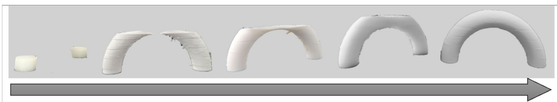
Fig. 10 Arch with constructed freeform printable layers with the M-AM deposition process
