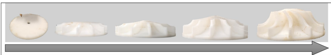
Fig. 11 Turbine with constructed freeform printable layers with the M-AM deposition process
