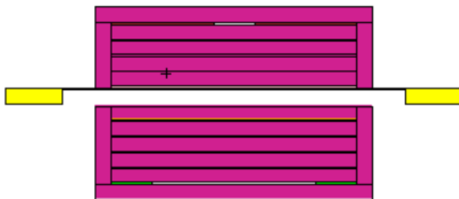
Figure 27: The separation of the TEX body at the platen. As the bottom half of the assembly moves on the lift, the separation changes.
