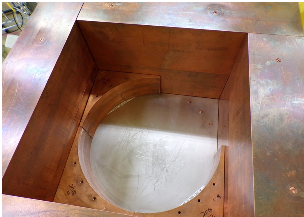
Figure 8: Example of the copper reflectors with the side reflectors and three corner reflectors installed.
