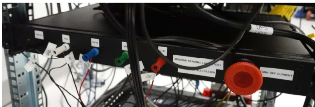
Figure 34. Argonne National Laboratory's custom 12-channel multiplexer for controlling electrochemical sensors in the Kairos test loop.
