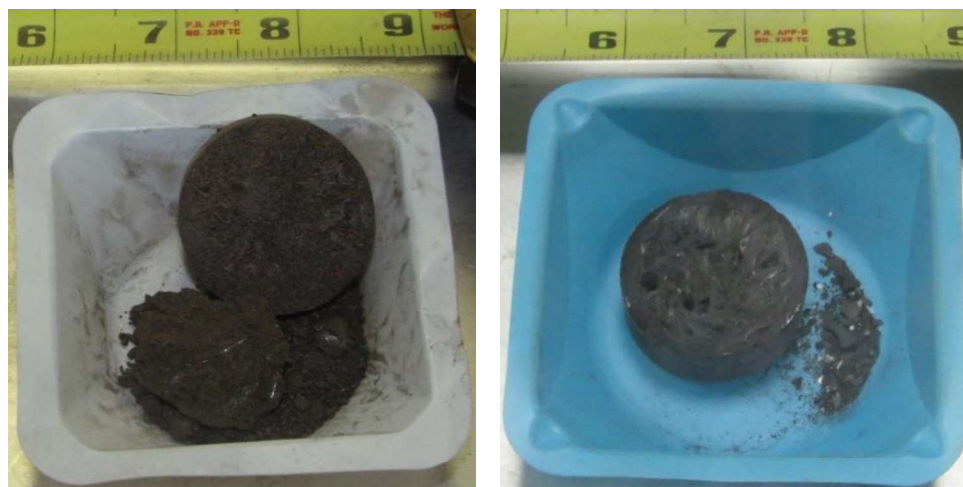
Figure 11. \text{LiCl-KCl-UCl}_3 (left) 72.3 wt% \text{UCl}_3 and (right) 60.8 wt% \text{UCl}_3 before and after electroanalytical experiments.
