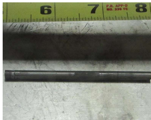
Figure 30. Depleted uranium-zirconium-molybdenum fuel rod used for salt processing studies in the MFIT
