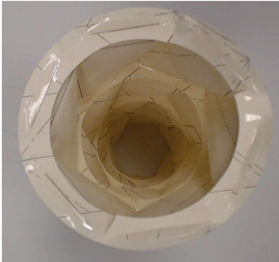
Figure 3-11. Deployed configuration of the bistable baffle assembly, axial view
