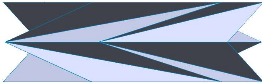
Figure 2-4. Deployed Kresling pattern, n=6 , folded into a 3d assembly, side view
