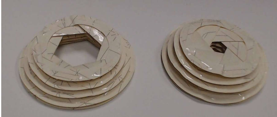
Figure 3-8. Stowed configuration of two baffle designs, stable 1/1/1.732 ratio on the left, bistable 1/1.5/1.9605 on the right
