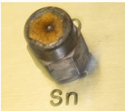
Figure 4: A tin (Sn) anode showing pitting and discoloration of the anode surface caused from prolonged exposure to high a voltage e- beam.
