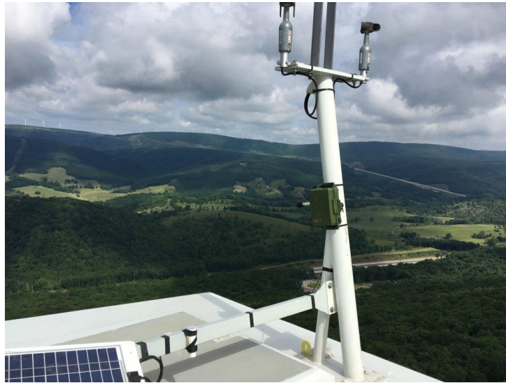
Figure 2.4. Photo of acoustic bat detector (in green box) mounted on the nacelle of Turbine 1 at the New Creek Wind Project, 2017.
