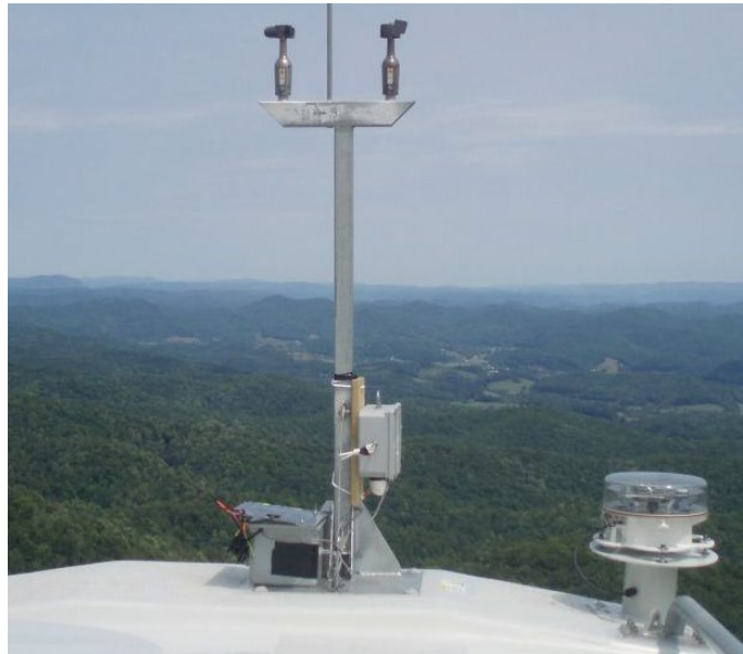
Figure 2.3. Photo of acoustic bat detector (in gray box) mounted on the nacelle of Turbine 47 at Laurel Mountain, fall 2011.
