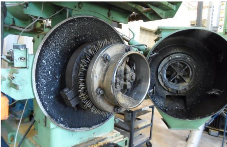
Pelletizing head open. See the pencils sticking out of the die.
