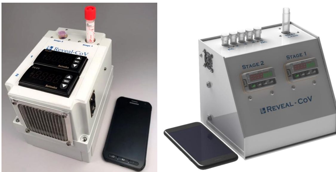
Figure 1. Reveal-CoV instrument development. Left: First unit build of prototype single assay instrument consisting of two single-tube heaters for sample inactivation (Stage 1) and detection assay amplification (Stage 2). Right: CAD model of 5 assay instrument concept consisting of a sample inactivation heater (Stage 1) and a 5-tube detection assay heater (Stage 2).
