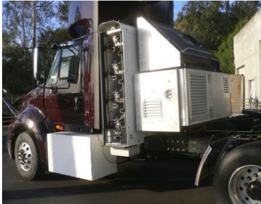
Figure 16: The prototype TransPower truck, FC1, about to enter commissioning (shown here without the port side cover for the hydrogen storage)
