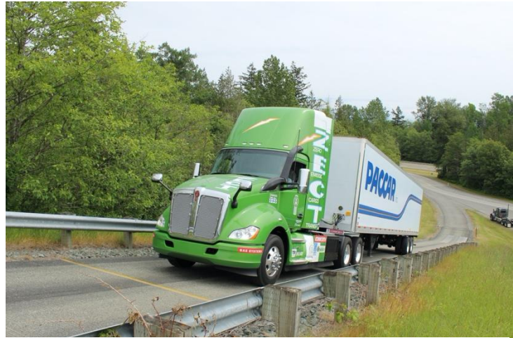
Figure 24. ZECT Climbing 30% Slope at 80,000 GVW
