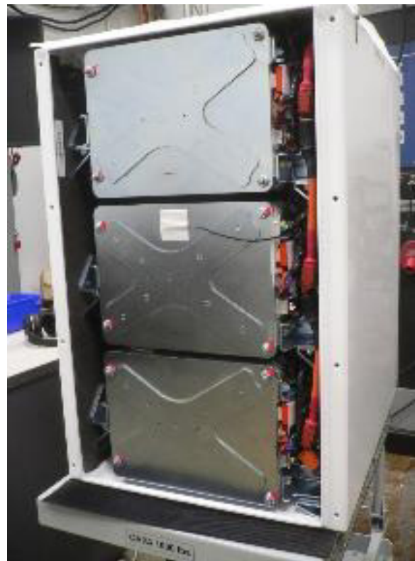
Figure 10 - One of four battery enclosures mounted to truck FC2, later retrofitted to FC1 as well, shown in test with front cover off.
