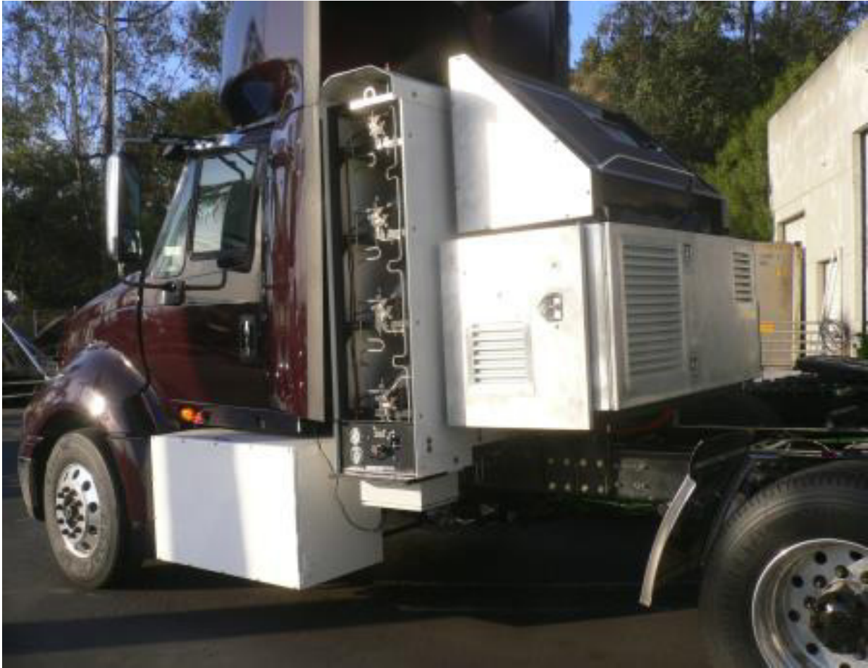
Figure 4-The prototype truck about to enter commissioning. Shown here without the port side cover for the hydrogen storage, showing the four tank valves which would all be replaced the following summer. The KAM cell batteries are under each door, the fuel cell APU is aft supporting the radiators.
