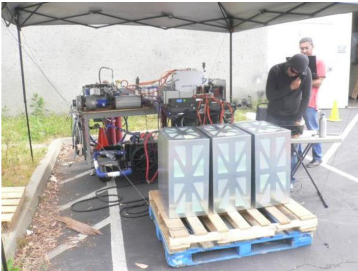
Figure 1-The benchtop fuel cell system was used to gain early experience with the HD30 fuel cell and with the required control processes. Batteries are on the skid in foreground, fuel cell at left under the tent, DC-DC highest at center. The large radiator for fuel cell cooling is largely obscured by the batteries.
