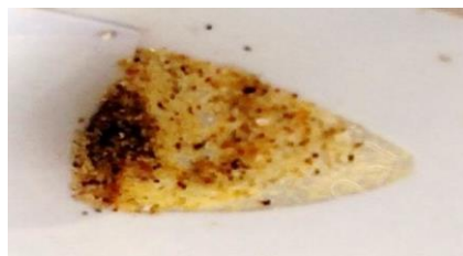
Debris from back-flushed condenser (sand and some rust)
