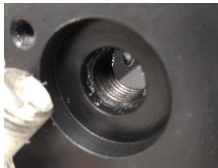
Threaded Connections – Coating Q/A Failed to Penetrate Thread
