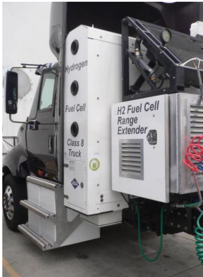
Figure 19: FC1, the prototype of the ZECT trucks, after being upgraded with NiMC storage batteries and the step structure shown below the cab
