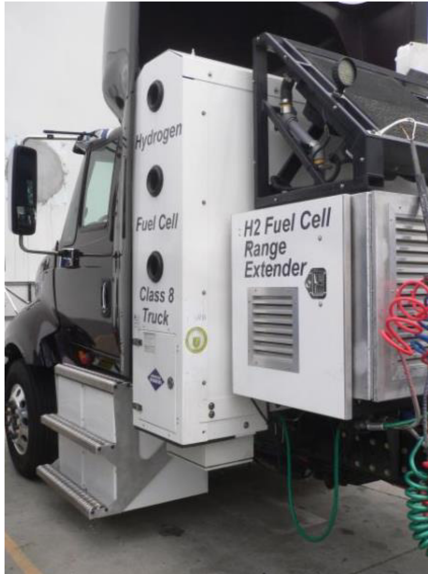
Figure 11- FC1, the prototype of the ZECT2 trucks, has been upgraded with NiMC storage batteries and the step structure shown below the cab.
