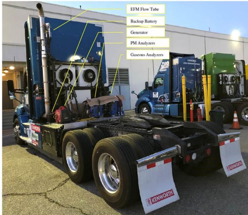
Figure 35 HECT truck with PEMS equipment installed
