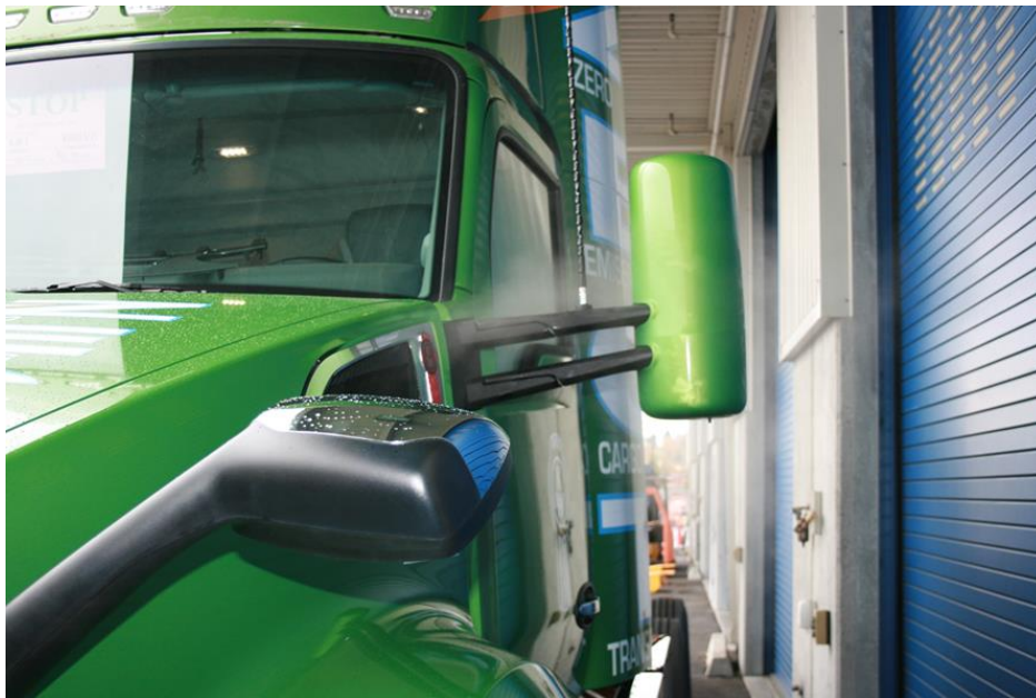
Figure 20. The water vapor from the fuel cell amassing on the driver windshield
