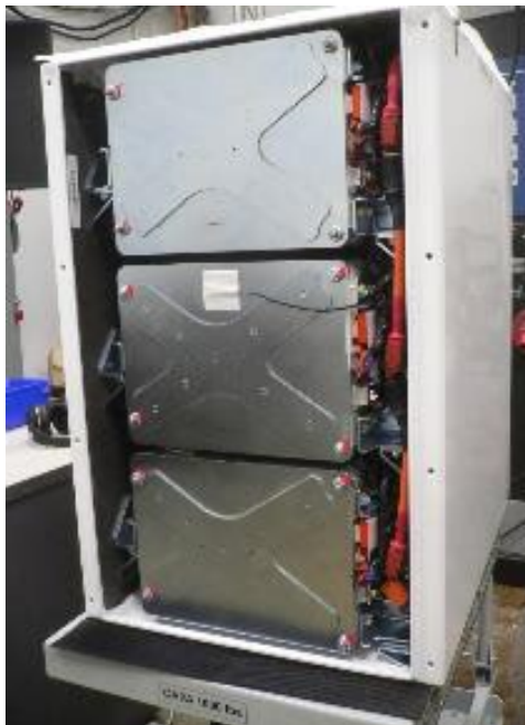
Figure 18: One of four battery enclosures mounted to truck FC2, later retrofitted to FC1 as well, shown in test with front cover off
