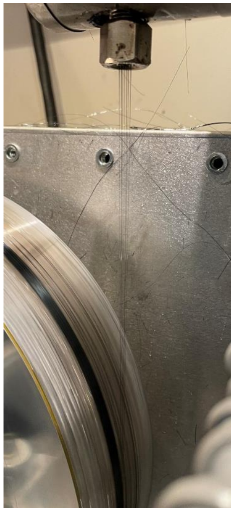
Figure 8. Lab-scale multi-filament spinning of pitch precursor tows. 7 filaments are simultaneously taken up onto a winder.
