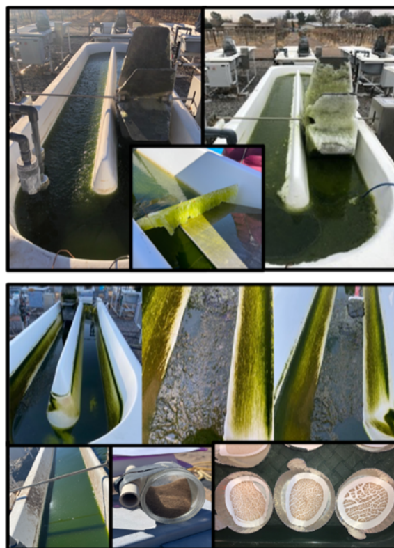
Fig. 2-7. Freezing conditions (top) and sediment accumulation due to high winds (bottom) in NMSU ponds.
