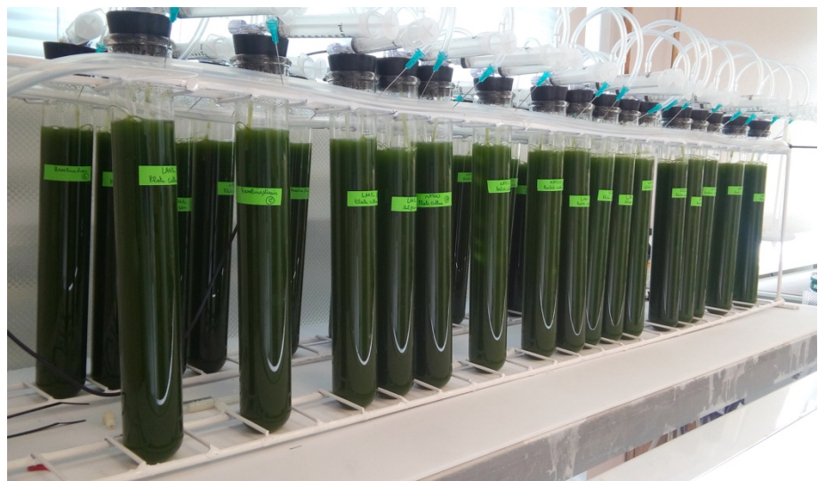
Fig. 3-2. Photo of the bubble column reactors used for the phenotype characterizations.
