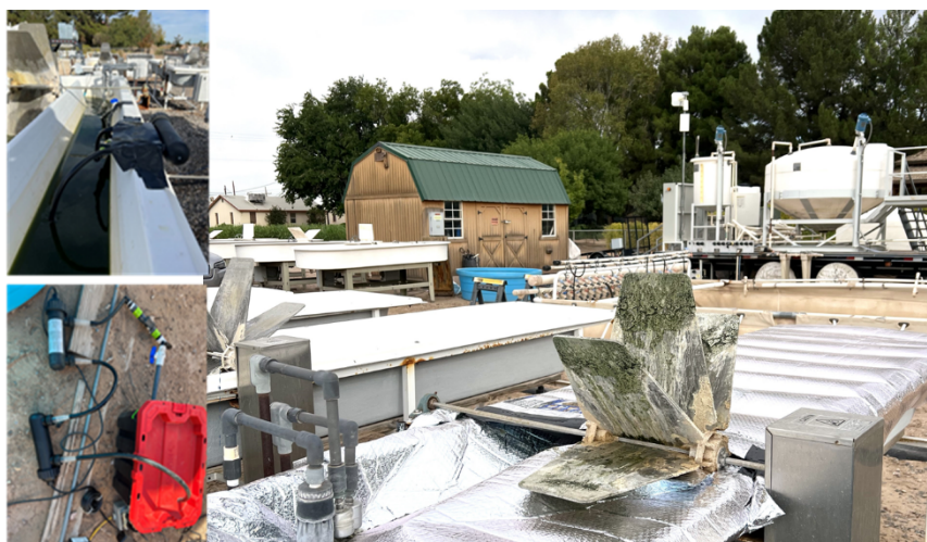
Fig. 5-7. Enhancements in Engineering and Process Execution for In Situ Field Applications. Illustrated are progressive engineering advancements that resulted in an optimized outdoor UV treatment process. Through successive iterations, we achieved an increased kill rate in algal subsamples while concurrently minimizing DNA repair mechanisms activated by light exposure in the field setting.
