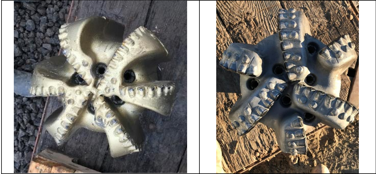
Figure 12. Bit 1 (left) and Bit 2 (right) used in the 12.25" interval.
