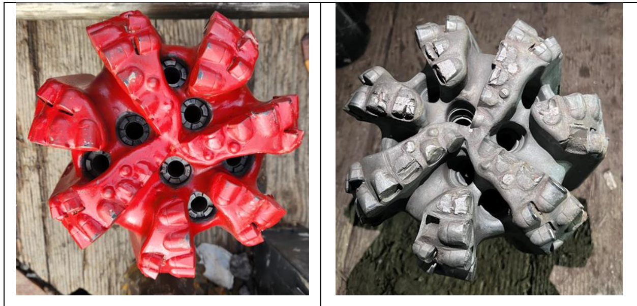
Figure 21. Bit 12 pre-drill (left) and post-drill (right) photographs.
