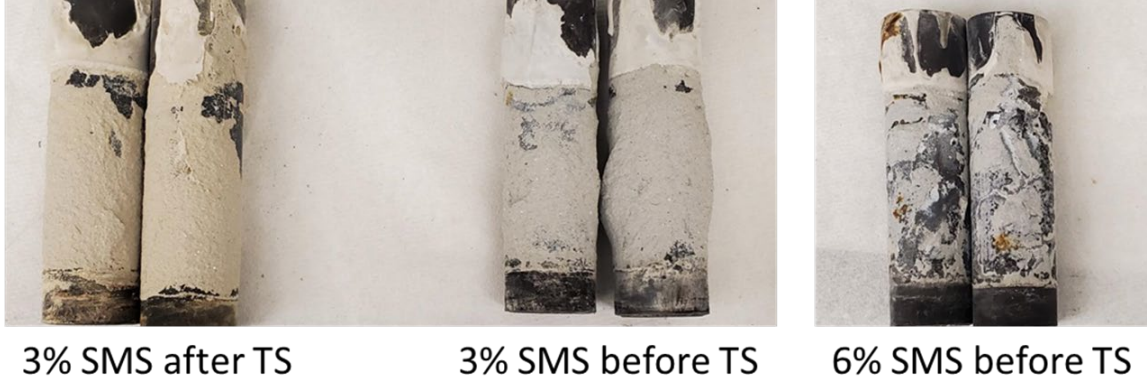
Figure 40. Appearance of carbon steel tubes after the shear-bond tests for TSRC samples with 3 and 6% SMS concentrations before and after the thermal shock tests.
