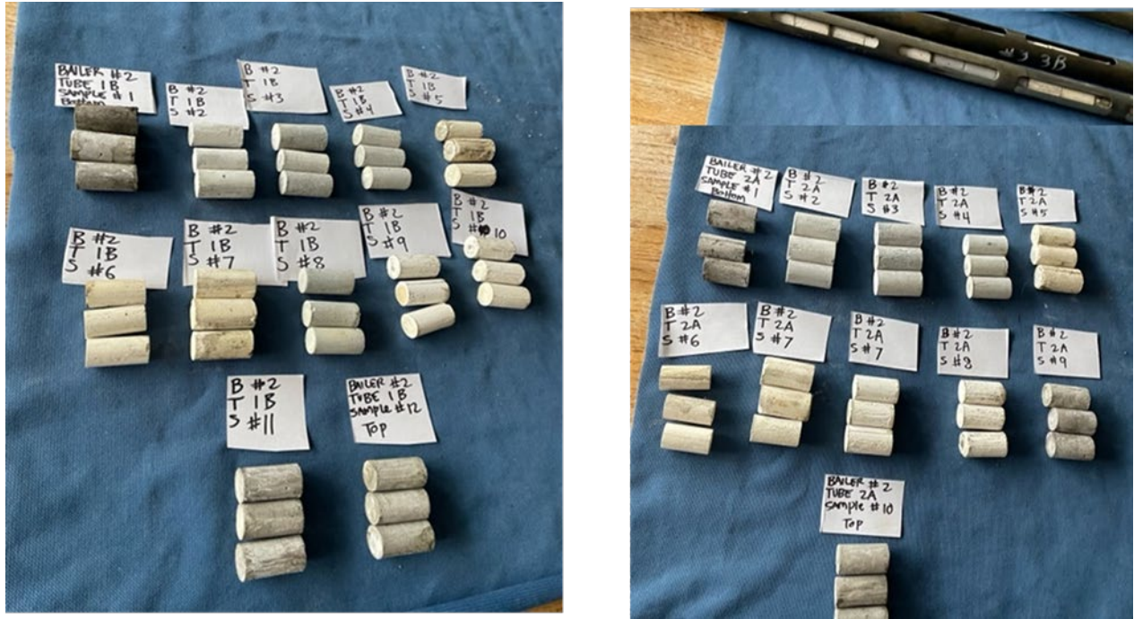
Figure 3: Photographs of the samples after the 3-month exposure in the Newberry well.
