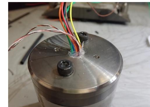
Wires sealed with RTV
