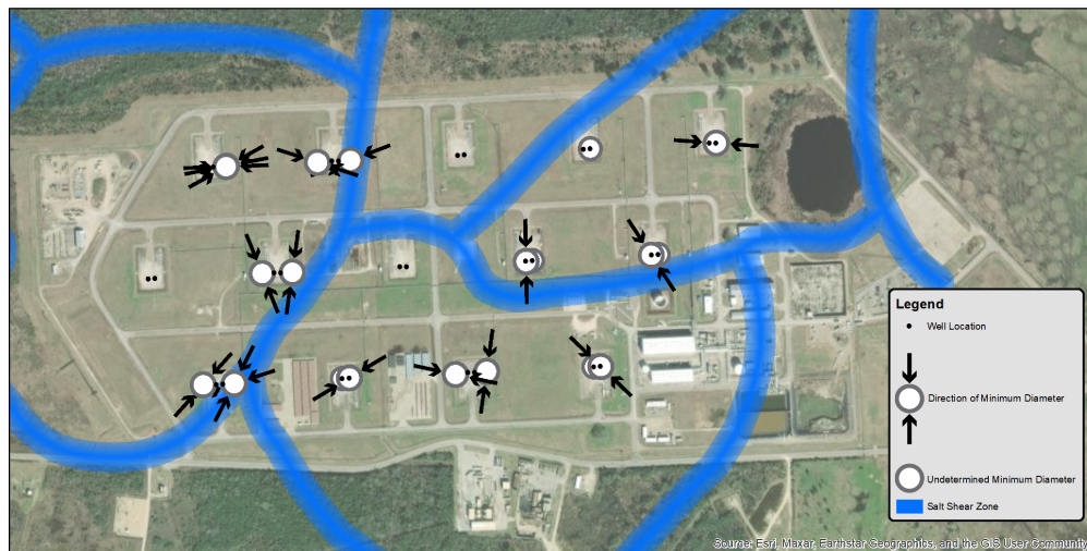
Figure 3-18. Comparison between salt shear zones and the orientation of minimum well diameter at the salt-caprock interface at the Big Hill site
