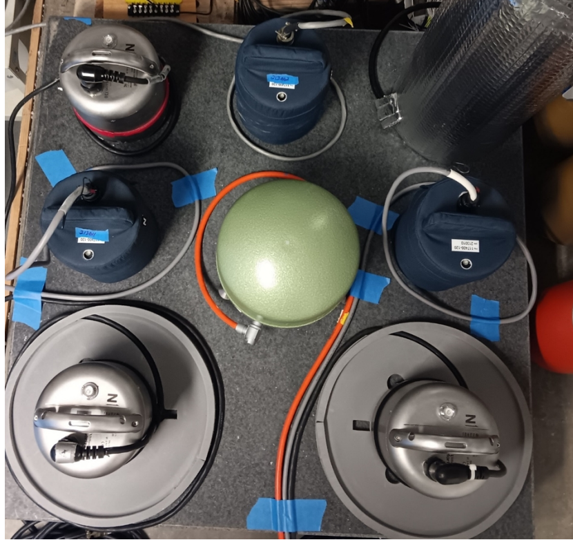
Figure 30 Sensors installed for Reference Frequency Response Test
