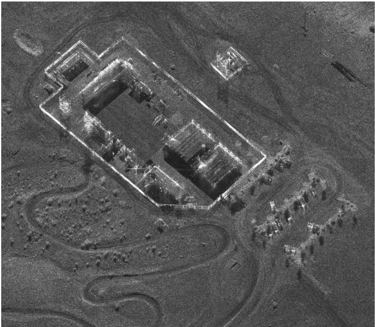
Figure 1. Example Ku-band SAR image of a Sandia National Laboratories test facility in Albuquerque, New Mexico, USA. Relevant parameters are 0.1016 m slant-range and cross-range resolution, nominal 6.858 km slant range, 30.3545 deg grazing angle, and -30 dBsm/m 2 noise floor.
