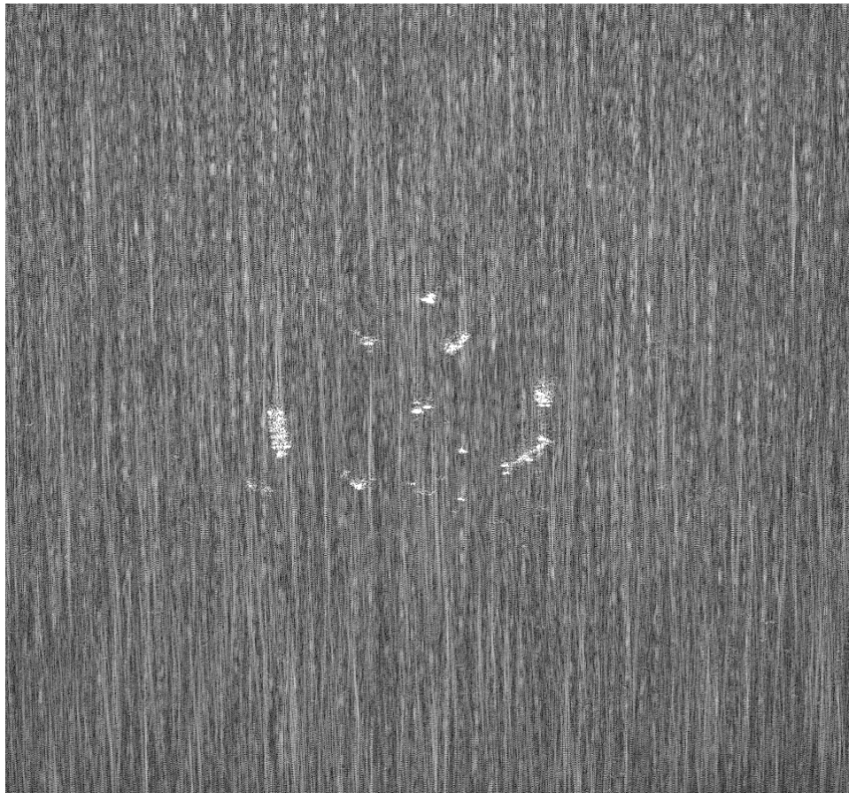
Figure 9. SAR image of a collection of vehicles imaged at L/S-band (2.16 GHz center) exhibiting 0.23-m resolution, corrupted by wireless digital service emissions.
