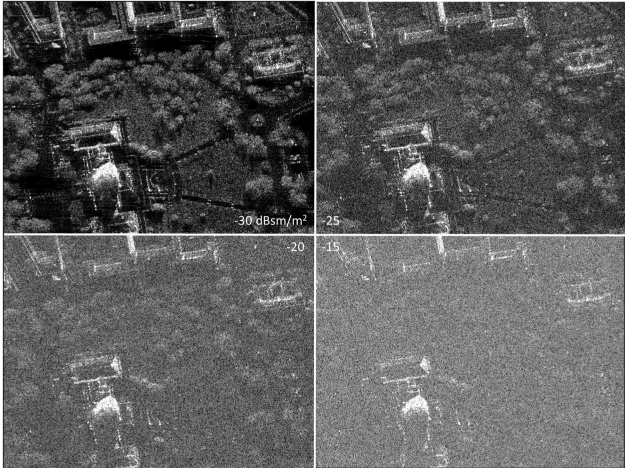
Figure 8. Ku-band SAR image of US Capitol building with various NER levels.
