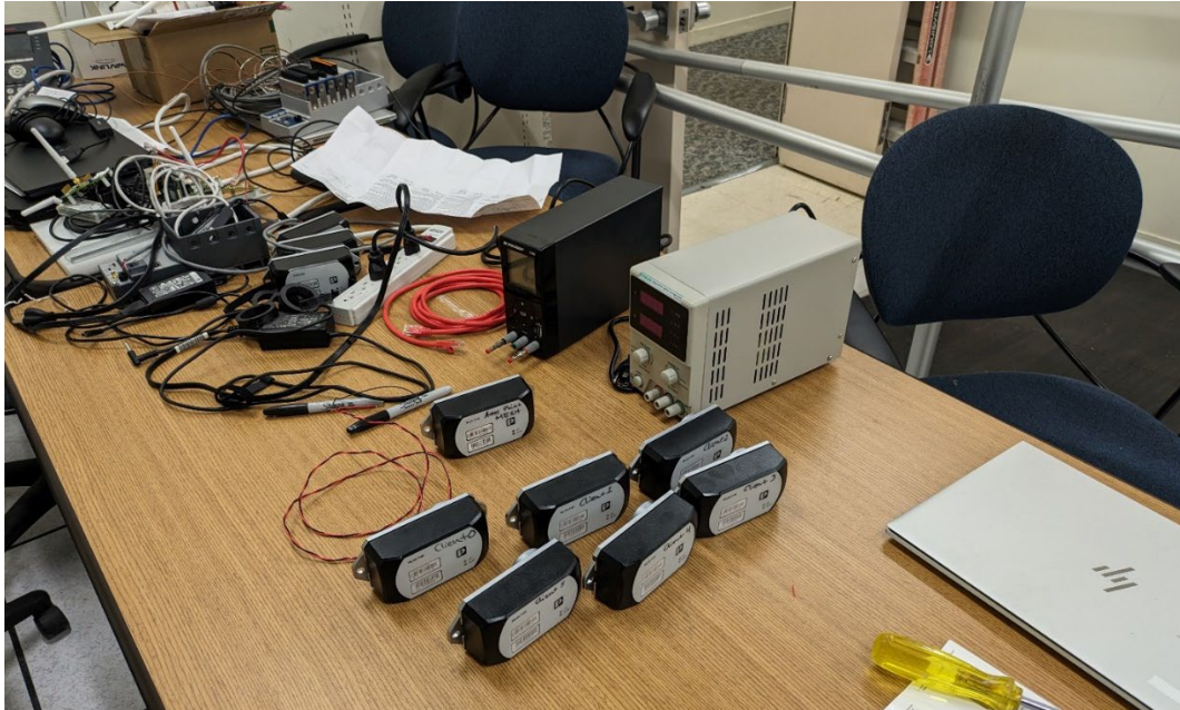
Figure 24. Benchtop Testing of Phoenix Contact 1100's and 2100 Pseudo-Mesh.
