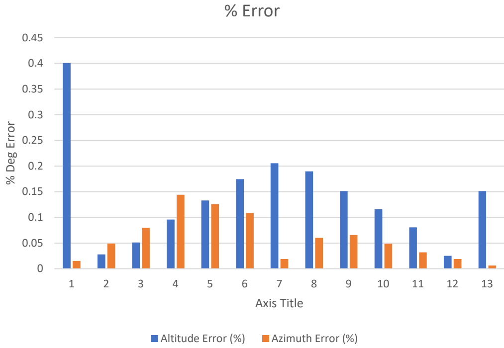
Figure 94. Sun Tracking Error of Old Sun Tracking Calculator
