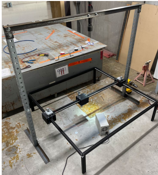
Figure 51. Small-scale, single heliostat closed-loop controls lamp test bed.
