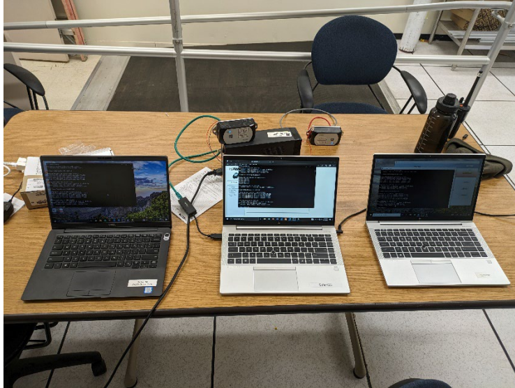
Figure 21. Wireless benchtop test setup for software and signal assessments with controller.
