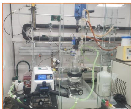
Figure 2. New modified continuous reactor for HOPI synthesis and the reduction in polymerization time with improved process.
