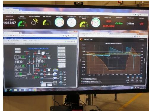
**Figure A.14:** Example image of a microgrid control interface.
