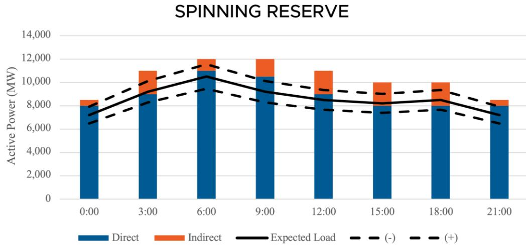
**Figure 4.2:** Conceptual expected peak system load, with uncertainty lines, along with available direct and indirect resources.
