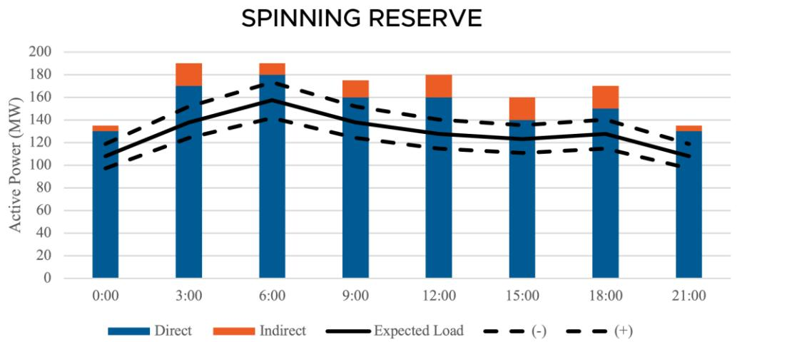
**Figure 4.1:** Spinning reserve, with uncertainty lines, along with available direct and indirect resources. In this case, the required spinning reserve, including maximum uncertainty, can be met with direct resources.
