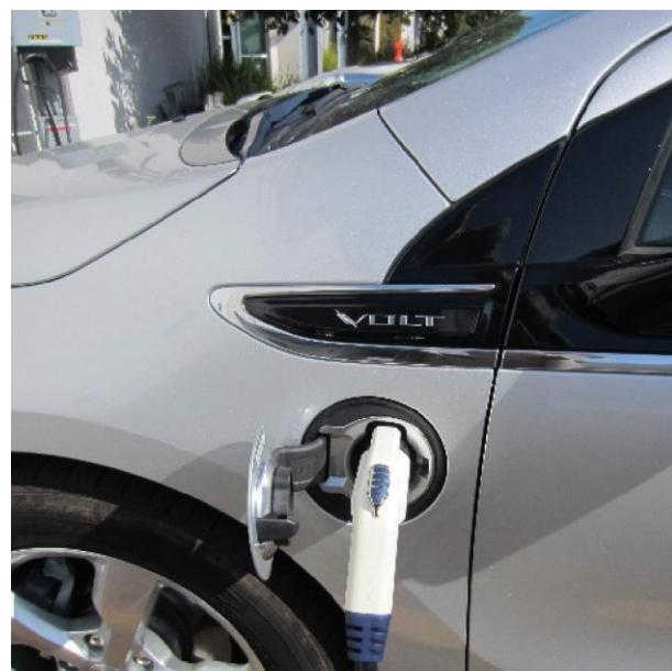
**Figure A.5:** Level 2 charging of an electric vehicle.
