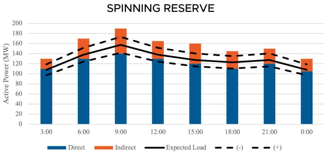
**Figure 4.3:** Spinning reserve, with uncertainty lines, along with available direct and indirect resources. In this case, the required spinning reserve, including maximum uncertainty, can be met with some level of indirect resources.
