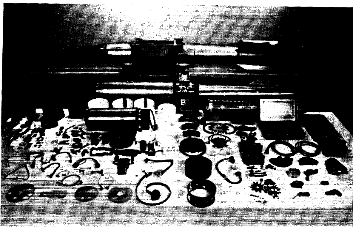
Figure 1. A B-61 nuclear bomb (rear) is broken down into four major sub-assemblies (center), which are dismantled separately (front).
