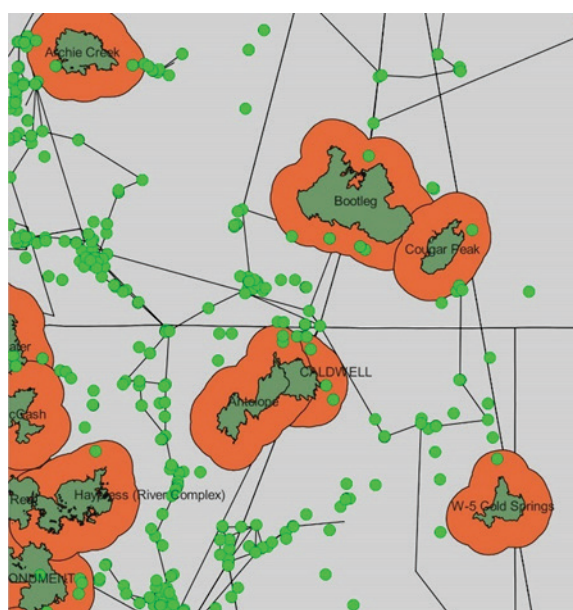
Figure 57. Bootleg, Cougar Peak, and Antelope wildfire fronts (in green) with offsets (in orange) to indicate assumed tripping of transmission lines due to heavy smoke and particulate matter.
