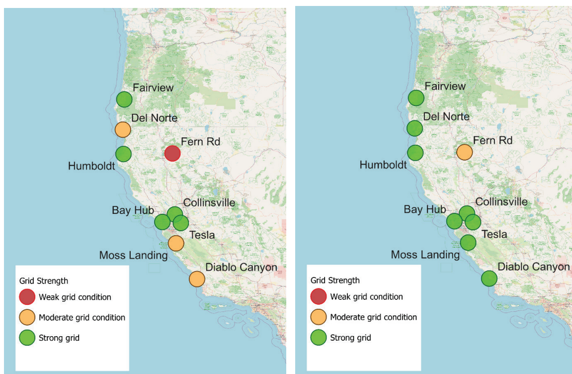
Figure 55. Grid strength visualization for the 2035 Distributed Topology for high offshore wind penetration scenario (left) without contribution of IBRs (right) considering short-circuit contribution of large IBRs (>100 MW)
