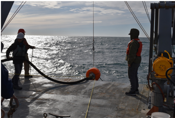
(c) The buoy trails behind as ship steams ahead, EM (d) With all mooring components except the MFN trail-cable and stretch hoses are fed aft, and buoyancy elements are transferred over the transom with the A-frame and released.
