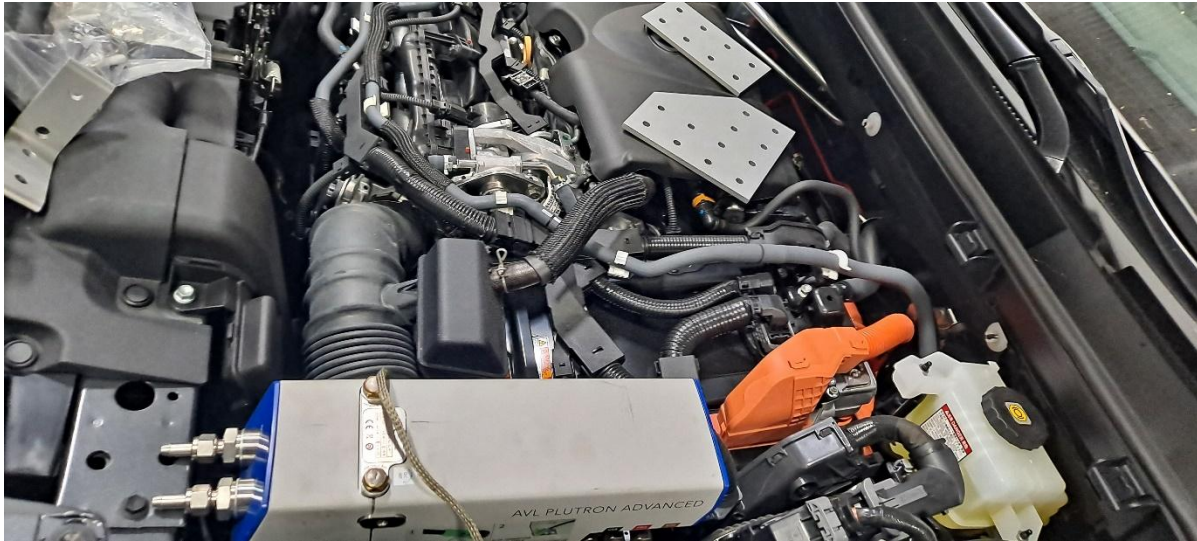
Figure 33: AVL Plutron Fuel Flow Meter installed on RAV4 in CAVE Laboratory
