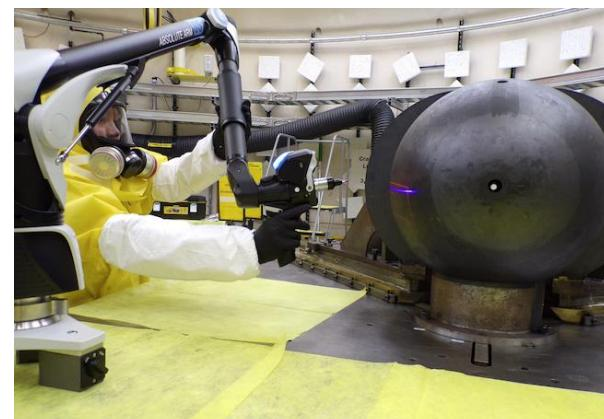
*Hot CMM measurements of the Flattop critical assembly natural uranium reflector to support a benchmark evaluation*
