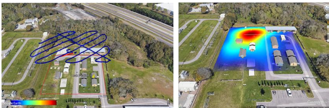
Figure 5: Methane concentration measurements using a UAV with a high sensitivity point sensor flying a horizontal grid pattern over the facility.
