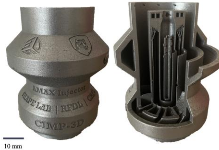
Figure 14. Final printed injector (left) with the cross-sectioned injector (right).
