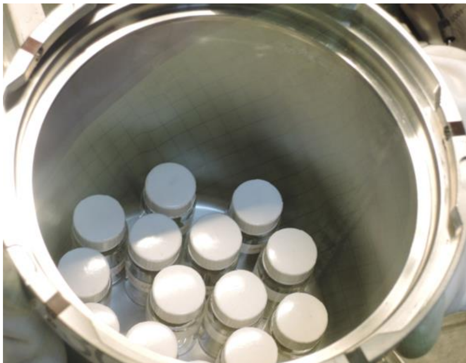
Figure 2. Experimental setup for stored \text{PuO}_2 samples analyzed by TGA-MS stored in a 3 quart SAVY-4000.
