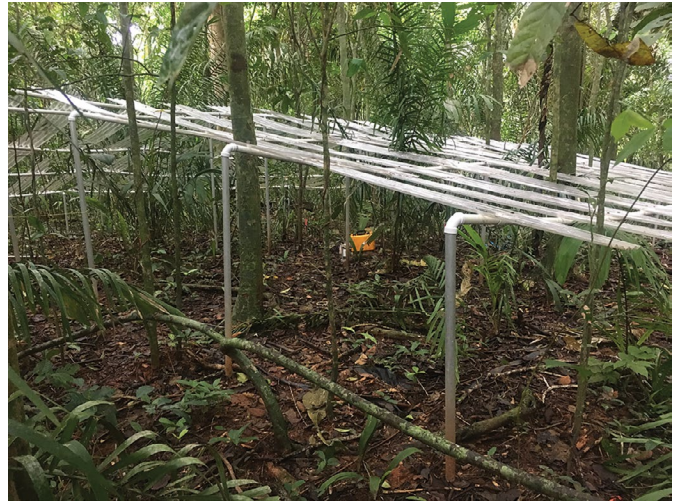
FIGURE 1. An example of one of the partial throughfall exclusion structures in the Panama Rainforest Changes with Experimental Drying (PaRChED), established in 2018 and diverting about 50% of throughfall away from 10 × 10 m plots ( n = 4 structures at each of 4 sites; 32 plots total including controls).
