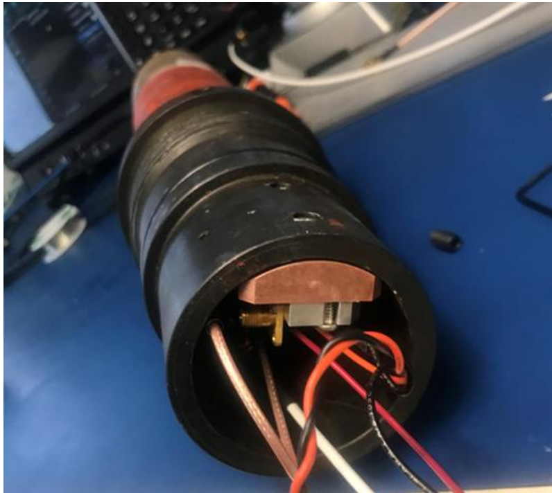
Figure 92: Copper Block Mounted to Metal Crossover for Enhanced Thermal Conductivity
