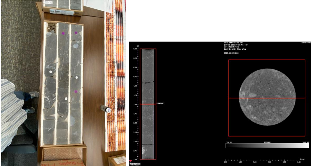
Figure 1b: Received core and log data and the CT scan of the full slab core.
