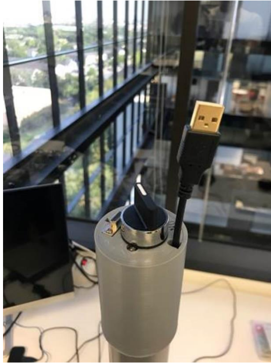
Figure 97: Top-End USB Access for Data Retrieval Without Chassis Removal
