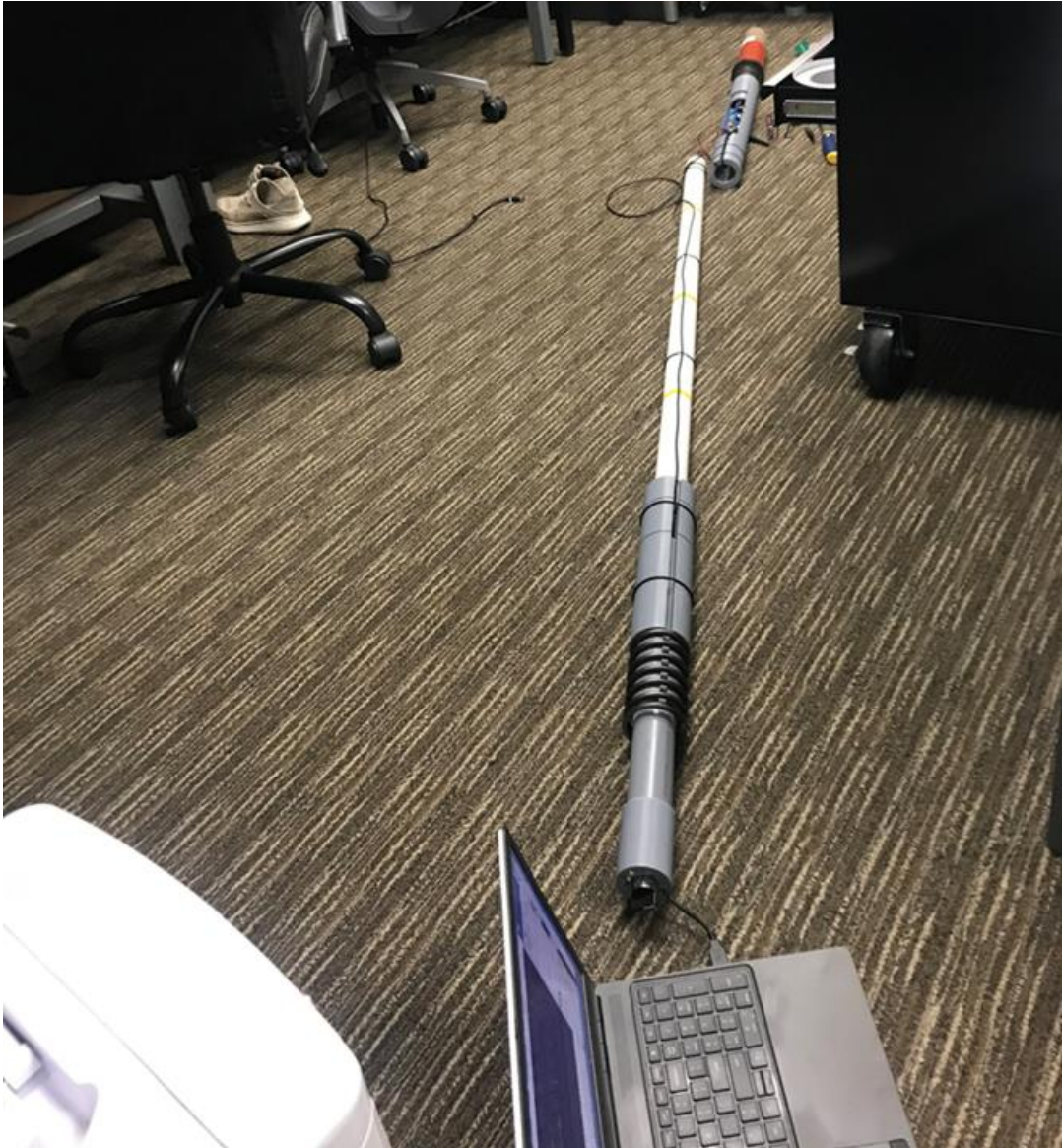
Figure 96: Fully Assembled System Powered by a 30V, 29Ah Lithium Battery with On/Off Switch
