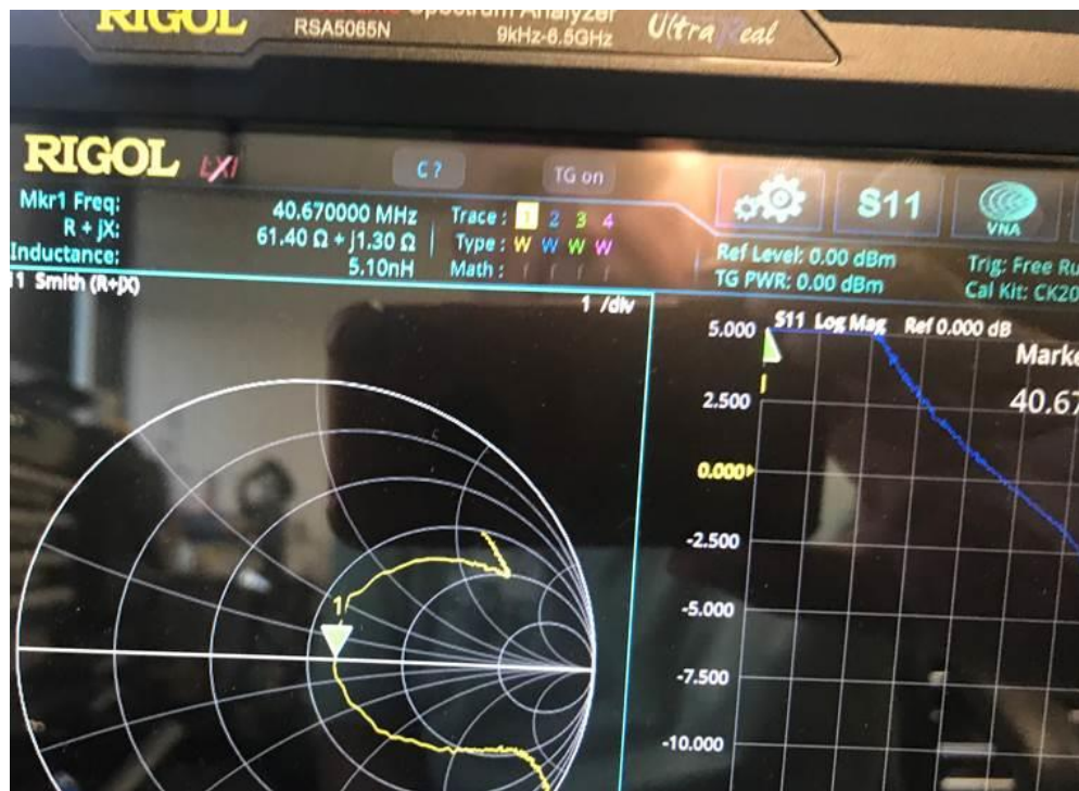
Figure 90: Transmitter Impedance Measurement and VSWR Tolerance Analysis with MOSFET Integration
