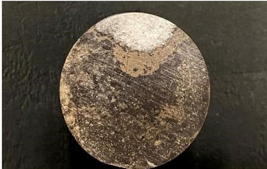
Figure 3: Anhydrite Nodule Within Dolomitic Paddock Formation Core Set 2- Sample ID 9, Depth 2597.40 feet
