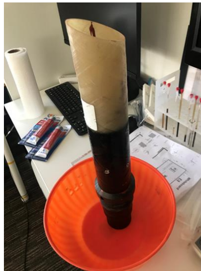
Figure 87: Fiber-glass housing Assembly with RTV Filling for Vibration Protection and Antenna Dielectric Matching
