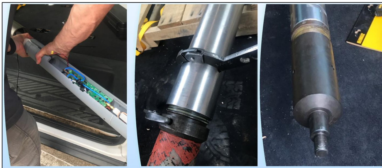
Figure 143: The chassis was loaded into the 3 5/8" pipe (left), and the lower cross-over was torqued in place with spanner wrenches. (the middle), and at the top-end, we provided another small sub with threads and o-rings that can be torqued in place and provide the final pressure seal. At the top of that sub is a thread whose profile was provided by EOG for attachment to the rope socket on slickline unit. (right)
