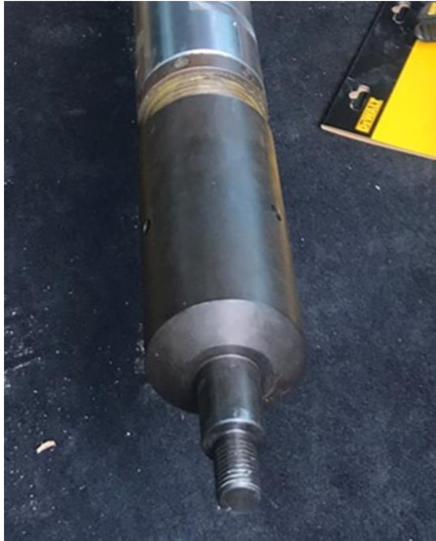
Figure 101: Top-End Subassembly with Threads and O-Rings for Final Pressure Seal and Rope Socket Attachment
