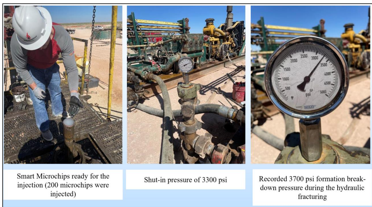
Figure 142: Smart Microchips ready for the injection (200 microchips were injected) (left), Shut-in pressure of 3300 psi (the middle), and Recorded 3700 psi formation break-down pressure during the hydraulic fracturing (right)
