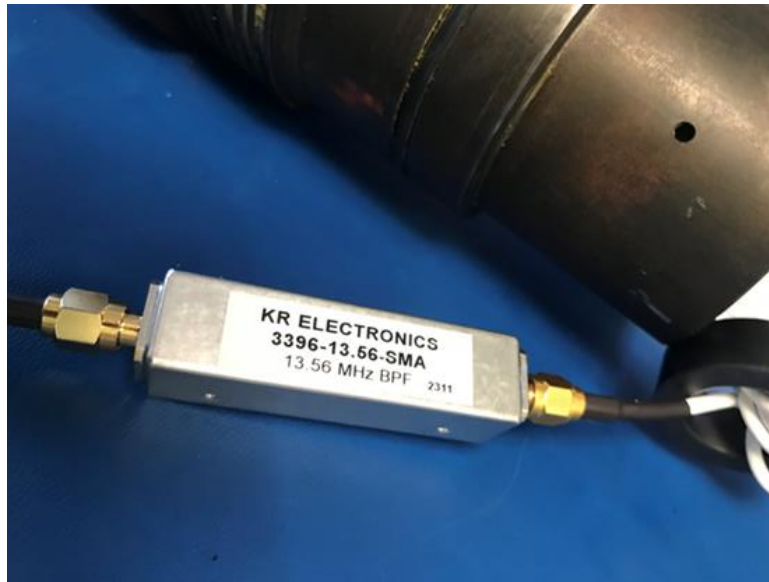
Figure 94: Addition of a 13.56 MHz Bandpass Filter for Signal Optimization
