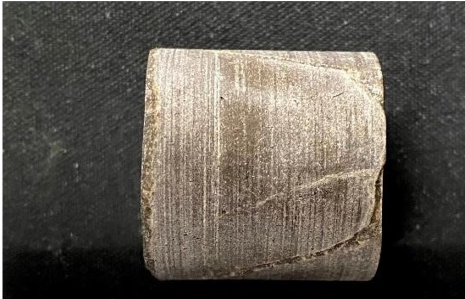
Figure 4: Paddock Core Sample Showing A Fissure or /Flaw In The Sample Core Set 1- Sample ID 7, Depth 2509.75 feet
