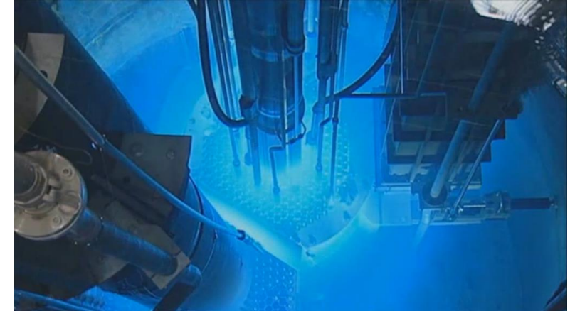
Photo of Sandia's ACRR Reactor. The blue glow is Cherenkov Radiation.
