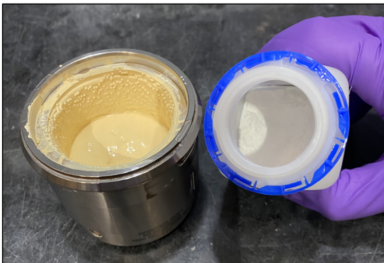
Figure A3: Picture of the ZnO:Zn, as-received, in the bottle (right) and after ball milling (left). The ball milled powder was a light-yellow color while the as-received powder was white.
