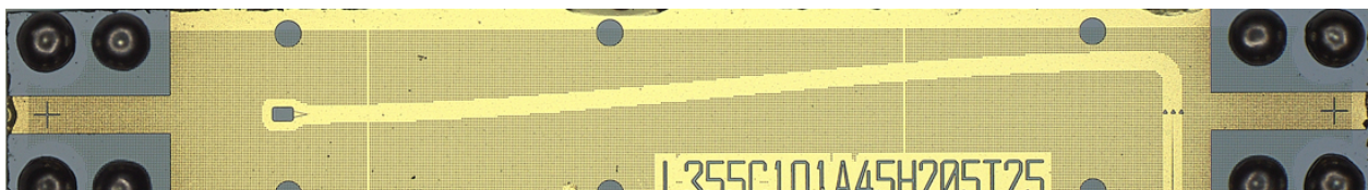
Figure 3: Optical image of the waveguide chip. On each end of the chip there are 4 solder pads (currently filled with solder) used for both registering the chip to the trap die and for attaching the waveguide chip to the trap. The input coupler of the chip is on the bottom right designed for free space coupling into the edge of the chip. The two alignment crosshairs are at the optical center of the chip at opposing ends.
