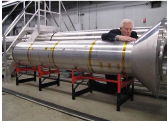
Figure 3-8. Hollow cylinder flare geometry. The figure is from Ref. [27].
